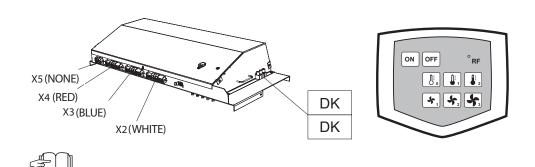
For detailed information of DM control modules installation into FINESSE air curtains read carefully: QUICK START manual for DM control modules installation (deliverot with control module)
