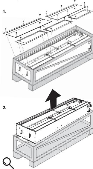
If the curtain has been transported at temperatures below 0° C, it will be necessary to let it sit for at least 2 hours under normal operating conditions after unpacking, without turning it on. This will allow the air curtain's interior te perature to stabilise.
